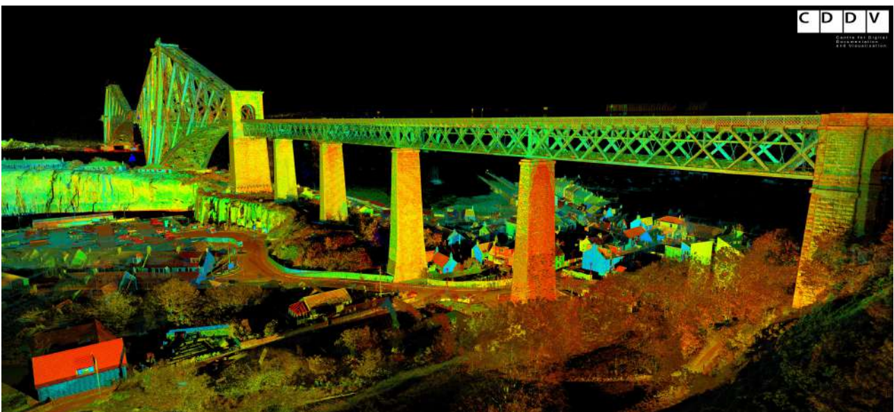
Image courtesy of CDDV, Point Cloud still from laser scanning of Forth Bridge, North Elevation 2016
